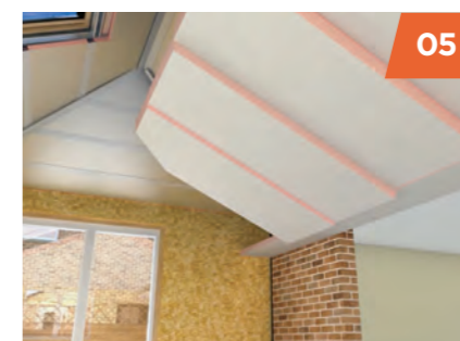
05 3 layers of high performance insulation (between and over rafters, and insulated plasterboard), is installed.
